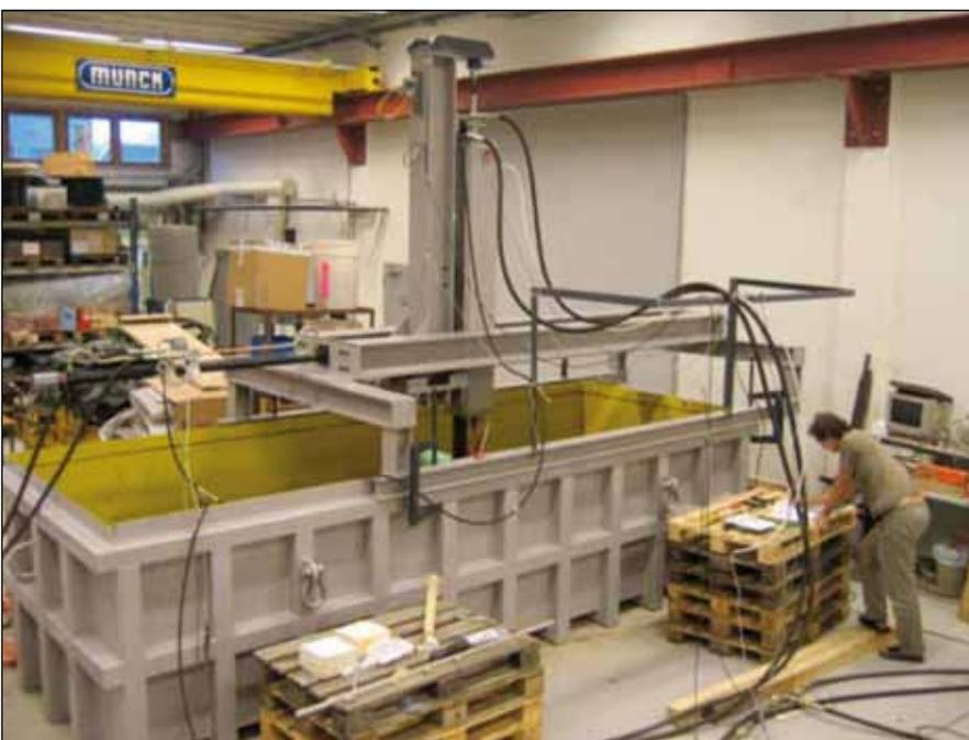
Large-scale pipe-soil interaction tests at NGI in Oslo.
