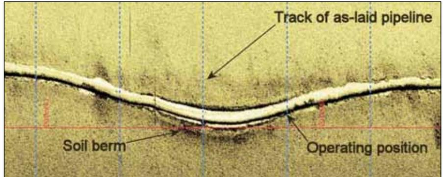
Lateral buckle from seabed side-scan sonar.
