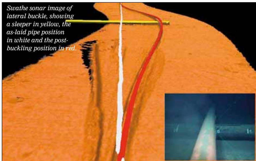
water, trenching and burying is less practical and with the higher pressures and temperatures often experienced in deepwater developments, this solution simply does not work. So what we now do is deliberately encourage the pipeline to buckle, but in a controlled way. By controlled initiation of lateral buckles at regular intervals, the loads are shared and reduced at each buckle site.
