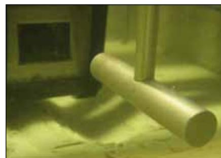
*Small-scale pipe-soil tests in the centrifuge at the University of Western Australia.*
